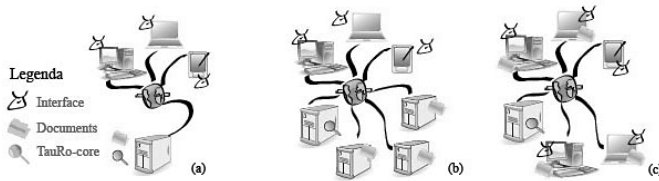
Figure 1 – Application scenario for TauRo-core: client-server (a), distributed (b), P2P (c).
